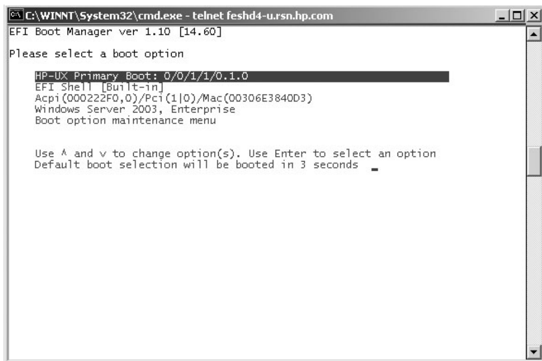
Figure 3-47 HP Integrity Superdome/sx2000 EFI Boot Manager
